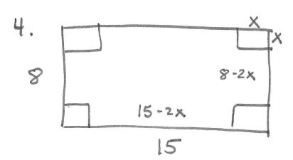
Maximize: V= lwh V = (15-2x)(8-2x)(x) $V = (120 - 46x + 4x^2)x$  $V = 120 \times -46 \times^{2} + 4 \times^{3}$ V' = 120 - 92 x +12x2 V'= 12x2-92x+120  $0 = 4(3x^2 - 23x + 30)$ 0 = 4(3x-5)(x-6)
